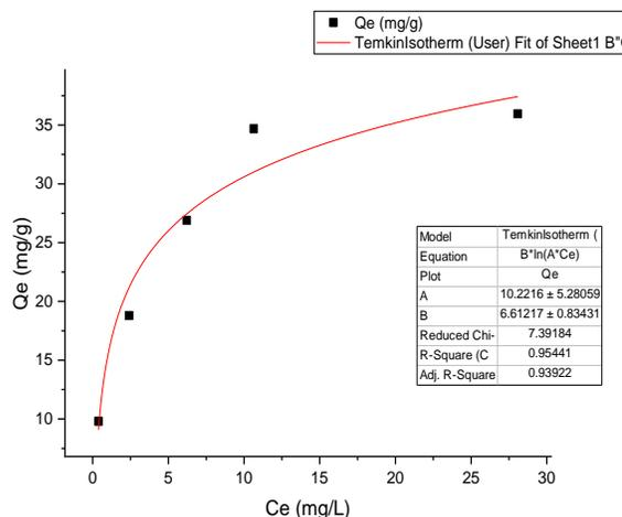
**Figure 10:** Temkin's adsorption isotherm for cadmium onto goat horn biochar
