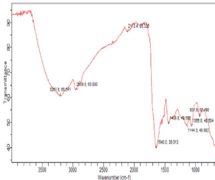
**Figure 1:** FTIR of goat horn biochar.
