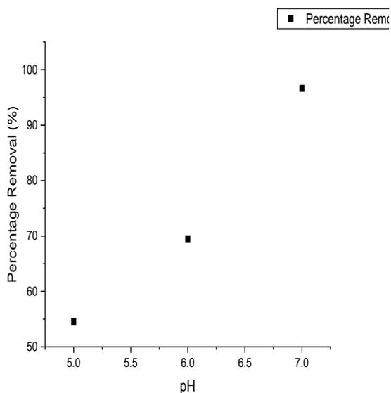
**Figure 5:** Effect of pH on percentage removal of cadmium ion on biochar
