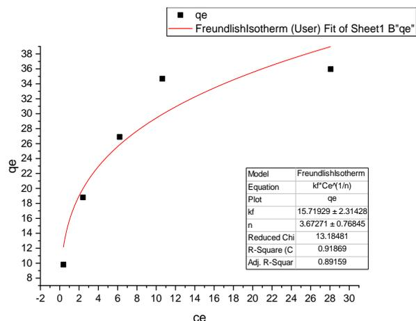
**Figure 9:** Freundlich adsorption isotherm for cadmium onto goat horn biochar
