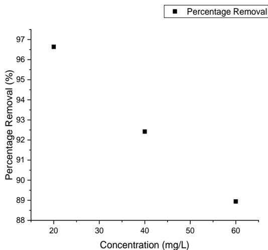
**Figure 6:** Effect of concentration on percentage removal of cadmium ion on biochar
