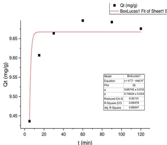
**Figure 11:** Pseudo First –Order adsorption kinetics of Cd ion on biochar.
