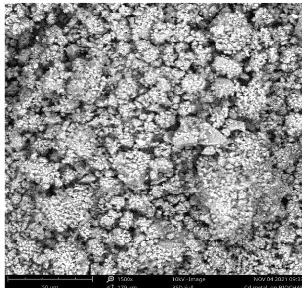
**Figure 4:** SEM image of Cd ion adsorbed on biochar.
