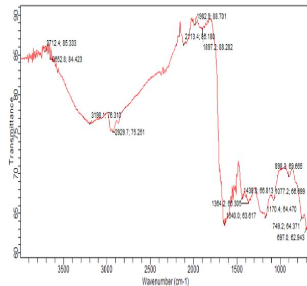
**Figure 2:** FTIR of adsorbed Cd ion on biochar
