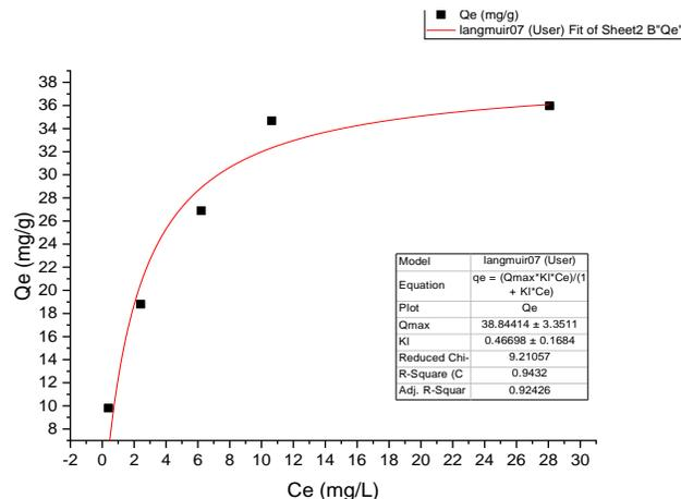
**Figure 8:** Langmuir adsorption isotherm for cadmium onto goat horn biochar
