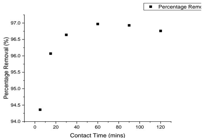
**Figure 7:** Effect of contact time on percentage removal of cadmium ion on biochar
