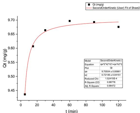
**Figure 12:** Pseudo second –Order adsorption kinetic for Cd ion on biochar.
