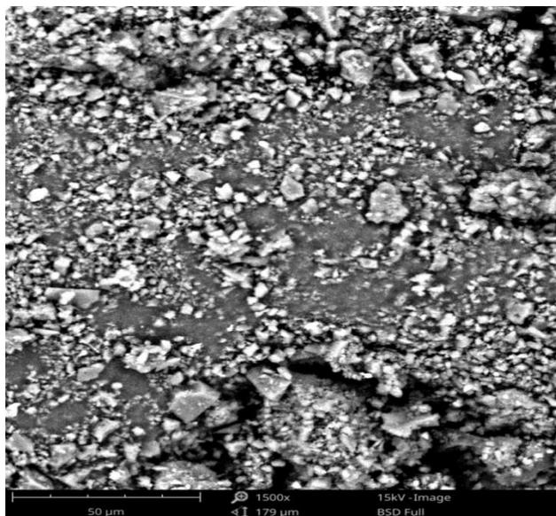
**Figure 3:** SEM image of the goat horn goat horn biochar
